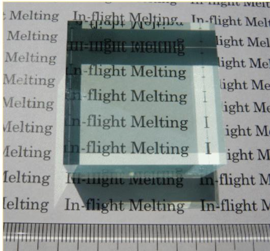
Fig. 10 In-flight melted glass block.
