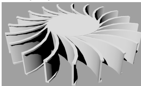
Fig. 18 Cycloid curve blade with opposite side fan (flow volume 4.24 l/sec)
