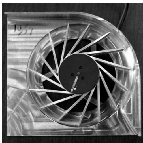
Fig. 10 Current fan (Thermal resistance 1.242 K/W)
