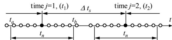
Fig. 3 Average with respect to time and definition of time interval.
