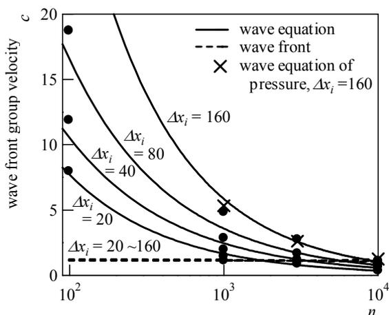
Fig. 15 Relation between propagation velocity of wave of disturbed velocity and space and time averages.
