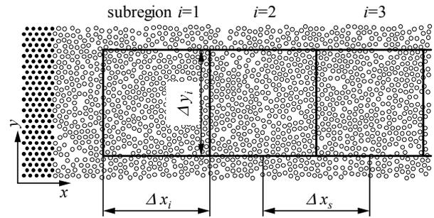
Fig. 1 Particles near the left end of the MD system and definition of subregion.
