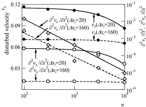
Fig. 9 Maximum values of disturbed velocity  $v_x$  and its derivatives  $\partial^2 v_x / \partial x^2$  and  $\partial^2 v_x / \partial t^2$  vs. number of averages.
