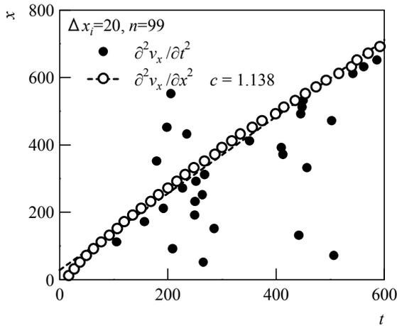
Fig. 10 Position of wave front (for the case of small amount of average) as changed with time.
