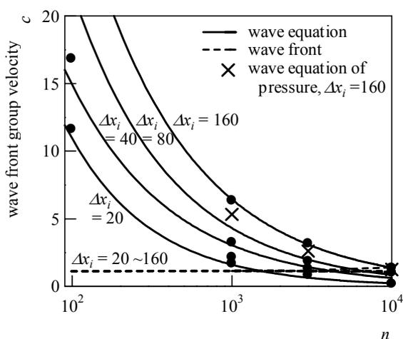
Fig. 16 Relation between propagation velocity of wave of disturbed density and space and time averages.
