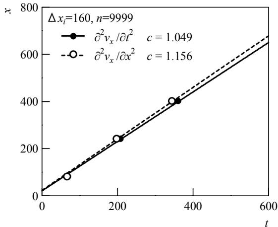
Fig. 11 Position of wave front (for the case of large amount of average) as changed with time.
