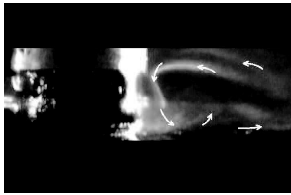
Fig. 17 Side view of the particle pathline in the experiment under heat gain with partition disk (Integrated, \Delta T_a^* = 0.81 , \Delta T = 7.6 [K]).
