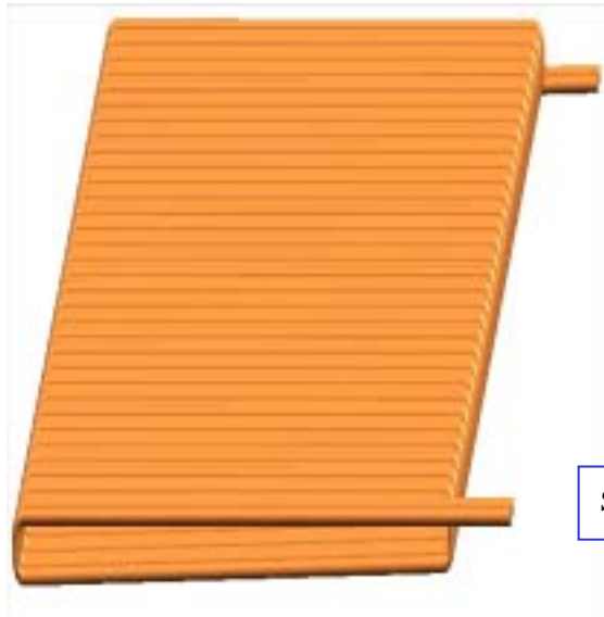
Fig. 12 Refrigerant side tube shape
