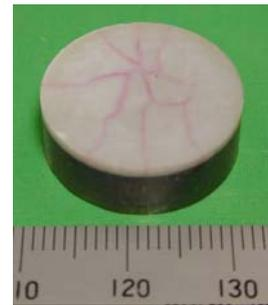
Fig. 9 Cracks on the ceramic surface of the alumina/nickel FGM disk.
