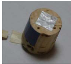
Photo 4 Probe for measuring surface temperature
