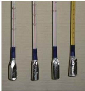
Photo 3 Mercury/ alcohol thermometers with radiation shields
