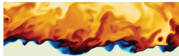
Fig.6 Instantaneous temperature field at  $Re_\tau = 550$ . The blue and red contours denote the low and high temperature regions, respectively.
