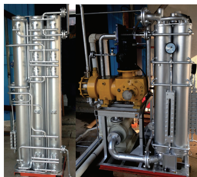
Fig. 19. Ammonia-water absorption freezer driven by diesel engine exhaust (Du et al., 2017).
