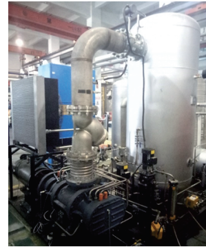
Fig. 16. The water vapor compression HP prototype for high temperature application.
